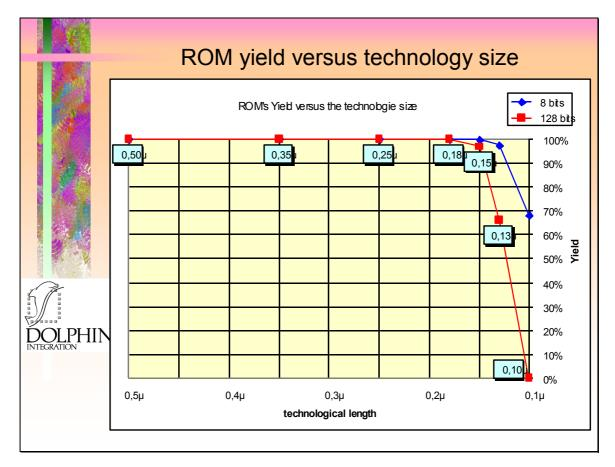
You can easily compute the effect of transistor matching on the yield of a ROM memory generator when you consider that one of the more sensitive cells of a memory is the read amplifier. For a given read margin, the yield will decrease when the offset will increase.
